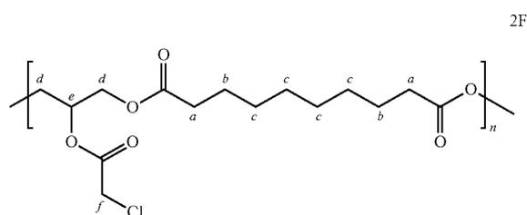
Compound 2F:  $^1\text{H NMR}$  ( $\text{CDCl}_3$ , 400 M)  $\delta$  5.25-5.35 (m, He), 4.11-4.49, (m, Hd), 4.07 (s, Hf), 2.31 (t,  $J=7.2$  Hz, Ha), 1.58-1.62 (m, Hb), 1.25-1.29 (m, Hc); FTIR (thin film)  $\nu_{\text{max}}$  2926, 2855, 1736, 1164, 786  $\text{cm}^{-1}$ .
