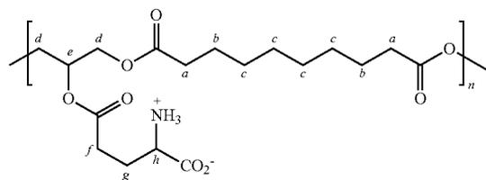
Compound 2B: <sup>1</sup>H NMR (MeOD-d<sub>4</sub>, 600 M) δ 5.28-5.29 (m, He), 3.97-4.38 (m, Hd, h), 2.58-2.68 (m, Hg), 2.35-2.40 (m, Ha), 2.17-2.28 (m, Hf), 1.62 (m, Hb), 1.34 (s, Hc); ATR-FTIR  $\nu_{max}$  3467, 2929, 2855, 1733, 1417, 1132 cm<sup>-1</sup>.
