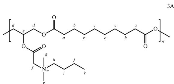
Compound 3A:  $^1\text{H NMR}$  ( $\text{DMSO-d}_6$ , 600M)  $\delta$  5.16-5.40 (m, He), 3.89-4.89 (m, Hdf), 3.50-3.57 (m, Hh), 3.35 (s, Hg), 2.27-2.33 (m, Ha), 1.64-1.69 (m, Hi), 1.48-1.51 (m, Hb), 1.27-1.32 (m, Hj), 1.24 (s, Hc), 0.92 (t,  $J=7.2$  Hz, Hk); ATR-FTIR  $\nu_{\text{max}}$  3383, 2931, 2856, 1736, 1167  $\text{cm}^{-1}$ .
