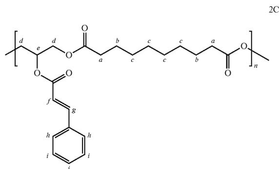
Compound 2C:  $^1\text{H NMR}$  ( $\text{CDCl}_3$ , 400 M)  $\delta$  7.69-7.74 (m, Hg), 7.54 (s, Hh), 7.41 (s, Hi), 6.43-6.67 (m, Hf), 5.25-5.43 (m, He), 3.38-4.52 (m, Hd), 2.30-2.33 (m, Ha), 1.59-1.61 (m, Hb), 1.27-1.29 (s, Hc); ATR-FTIR  $\nu_{\text{max}}$  3435, 2927, 2855, 1718, 1636, 1156, 982  $\text{cm}^{-1}$ .
