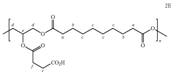
Compound 2E:  $^1\text{H NMR}$  ( $\text{MeOD-d}_6$ , 400 M)  $\delta$  5.27-5.32 (m, He), 4.17-4.40 (m, Hd), 2.61-2.62 (m, Hf), 2.35-2.39 (m, Ha), 1.62-1.65 (m, Hb), 1.35 (m, Hc); ATR-FTIR  $\nu_{\text{max}}$  2929, 2855, 1733, 1711, 1150  $\text{cm}^{-1}$ .
